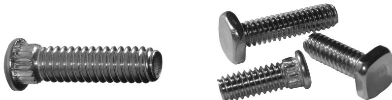
**Application:** The square head fits perfectly into most hurricane panel tracks. The hex head is a less expensive alternative to the square track bolt. The knurled studs are used in the studded angle tracks.
