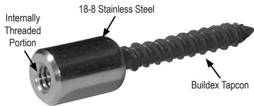
• **Application:** For use in concrete. Any length Tapcon® may be ordered. The stainless steel cap accepts a 1/4-20 bolt. Use a 3/16" masonry drill bit to predrill for the Tapcon®. Use a 9/16" masonry bit to countersink the 1/4-20 female portion and use the torx bit to drive the anchor.
